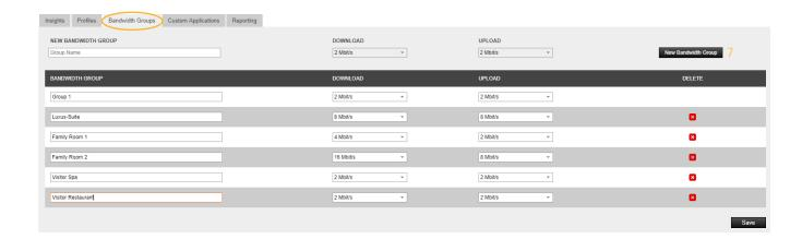
Configure new bandwidth groups by clicking on New Bandwidth Group<sup>7</sup>. Choose a meaningful name and assign the Down- und Upload Rate (this can be changed at any time). So not forget to save!
