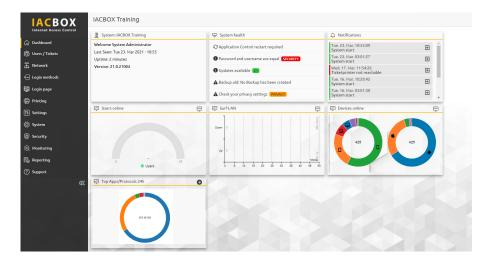
The arrow symbol takes you directly to the Application Control menu. After an hour, a diagram will appear. The relevance of the information displayed will increase after an appropriate period of time depending on the level of traffic on your IACBOX.
